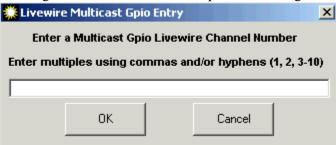
Once you have added the channel number you wish to use complete the router dialog to commit the new IOs into the router. Now these IOs can be used in stack events, standard events, and any other gpio capabilities in the Pathfinder system.
