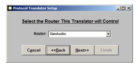
You must select the router in the system that this translator will use. It is recommended that virtual router be created with only the sources and destinations you wish to expose to this protocol translator in it. Then select that Virtual Router from the drop down list in the configuration for this protocol translator.
