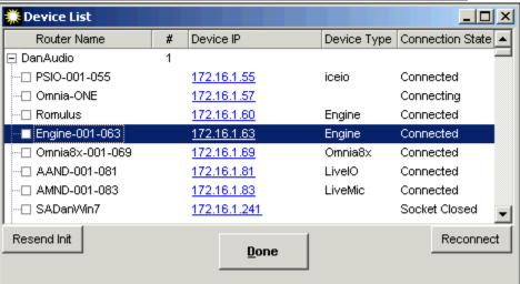
Please note that any device that does not have the device type listed within the first 60 seconds after the server launches should be tested for proper operation, as this is usually a signal that PathfinderPC Server cannot contact it properly. The logging and log files if configured can also supply more information.
